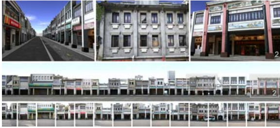
Figure 13: Image-based facade modeling [XFT*08]. 3D facades are reconstructed from multiple ground-level streetview images. The images are courtesy of Tan Ping, National University of Singapore, Singapore.
