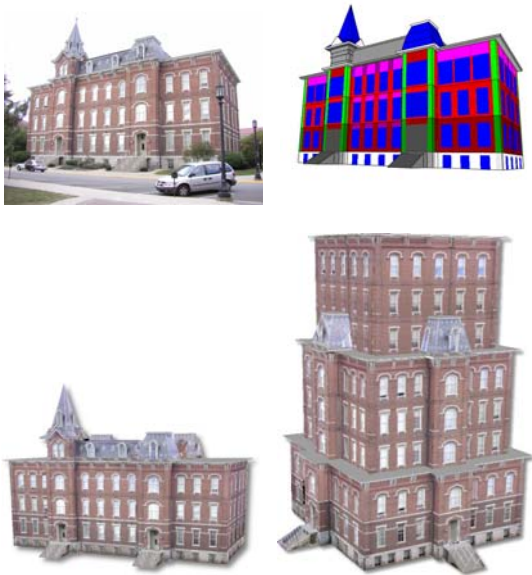
Figure 14: Style grammars for visualization of architecture [ARB07]. The user creates and subdivides an initial model of the building (top left). Repetitive patterns of the building features are automatically found and a representative grammar is constructed (top right). The user can then view the captured model (bottom left) and change the model on the fly producing new models (bottom right).
